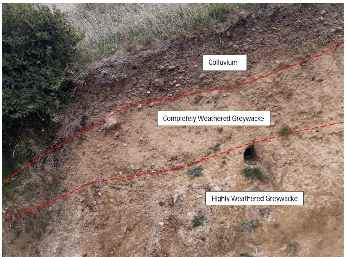
Photograph 4.5: Example of highly and completely weathered greywacke on the windfarm site
