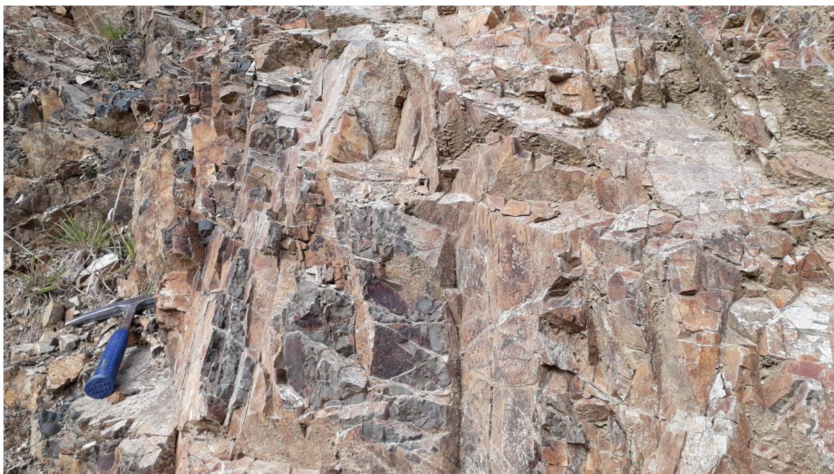
Photograph 4.4: Jointed moderately weathered greywacke rock typical of the windfarm site
