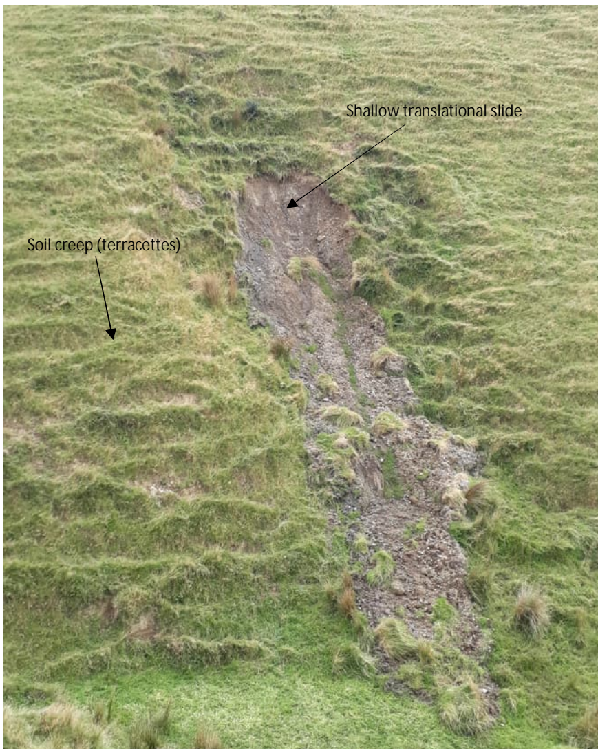
Photograph 4.11: Example translational landslide and shallow creep forming terraces (refer Geological Observations Plan in Appendix B for approximate location)
