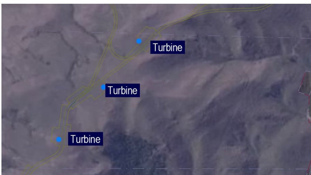
Figure 5.4: Typical turbine access via central wind farm road or spur road.
